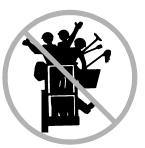
Do not exceed rated platform load capacity.
