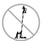
Do not move the machine while the platform is raised.
