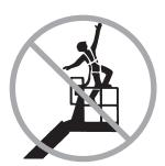
Do not sit, stand, or climb on the platform guard rails and Access Deck toeboard. Maintain a firm footing on the platform or Access Deck floor at all times.
