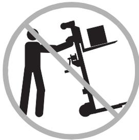
Do not move the machine with a raised load, except for minor positioning.
